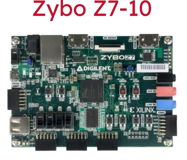
The Z7-10 includes a Zynq-7000 FPGA and 2 HDMI ports which make it perfect for testing passthrough through HDMI
